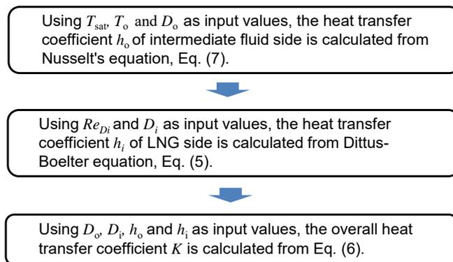
**Fig. 5 Condensation calculation flow on a single tube**
