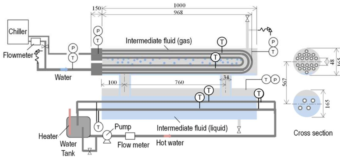
**Fig. 7 Tested laboratory scale IFV system.**
