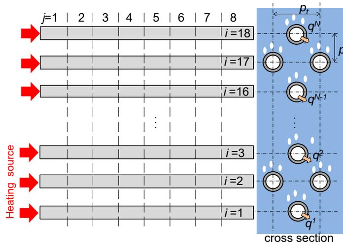
**Fig. 9 Segmented calculation model of tube bundle IFV evaporator**
