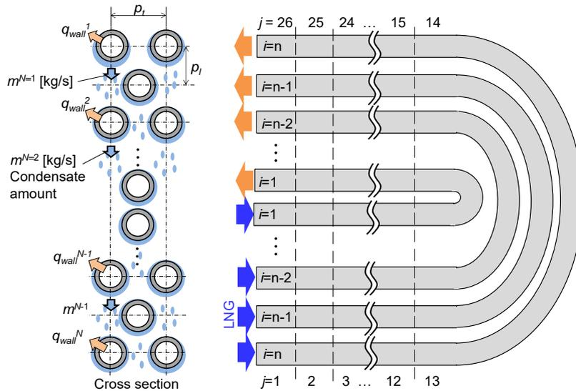
**Fig. 11 Segmented calculation model of IFV condenser**
