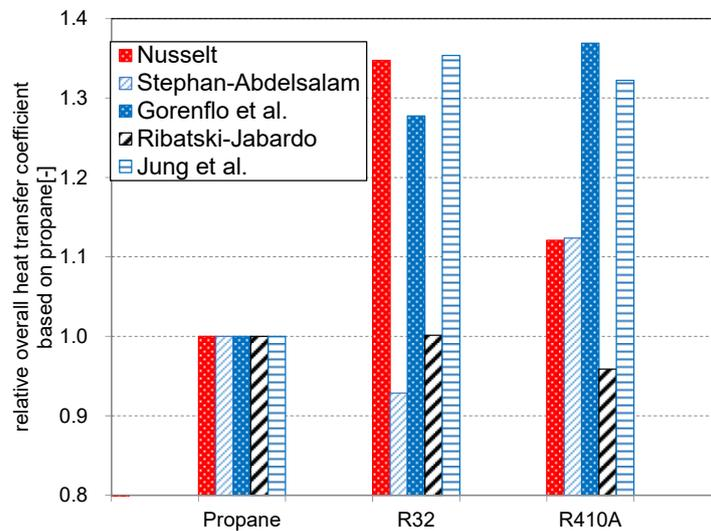
**Fig. 6 Predicted overall heat transfer coefficients on a single tube. (relative overall heat transfer coefficient using Nusselt Eq. (7) for condensation heat transfer coefficient; Stephan-Abdelsalam Eq. (1), Gorenflo et al., Eq.(2), Ribatski-Jabardo Eq.(3), and Jung et al., Eq. (4) for pool boiling heat transfer coefficient)**
