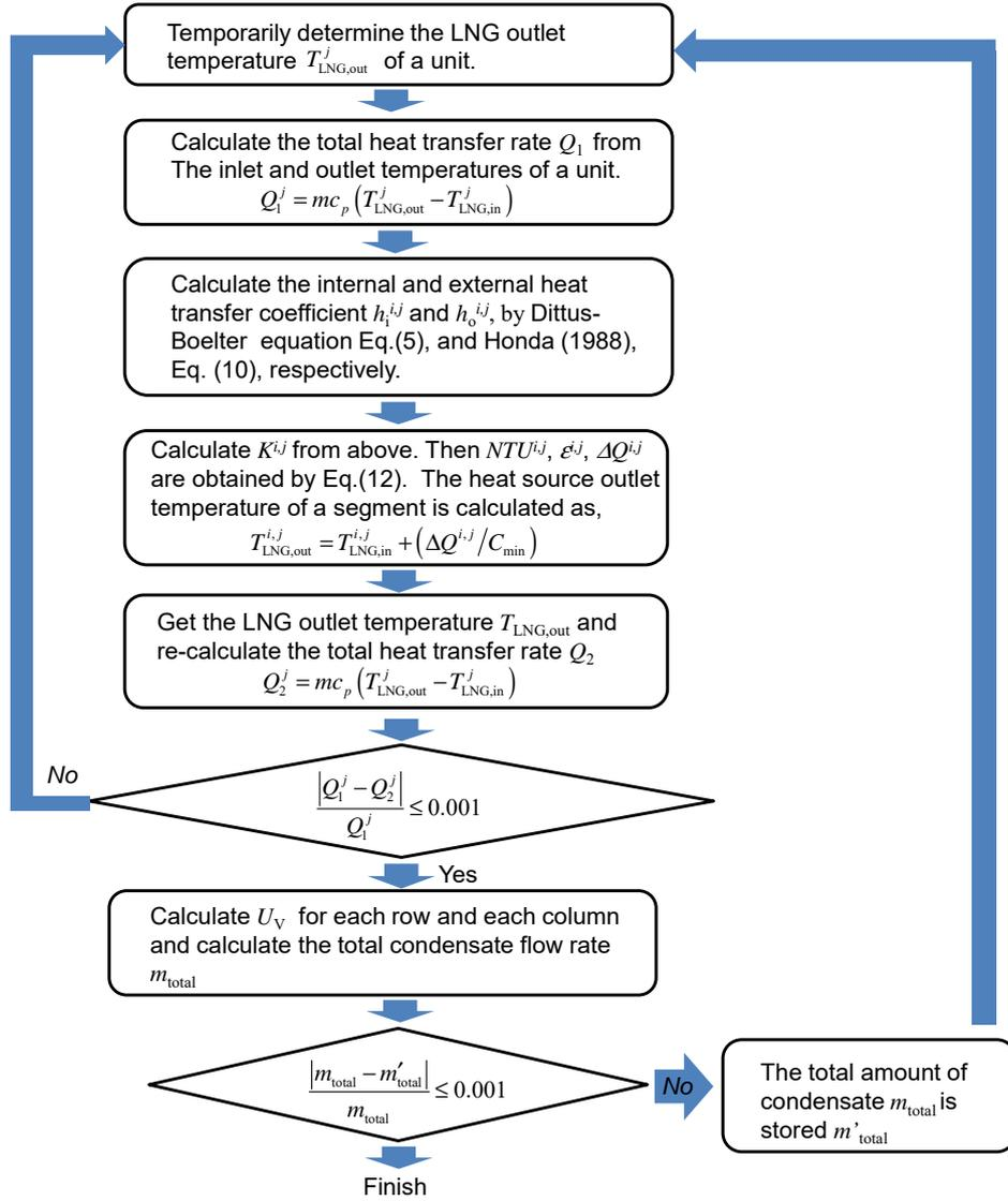
**Fig. 12 Calculation procedure for condenser**
