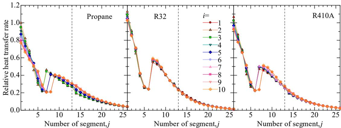
**Fig. 14 Heat transfer rate profile in condenser**
