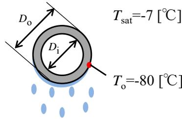
**Fig. 4 Condensation model of a single tube (Stainless)**
