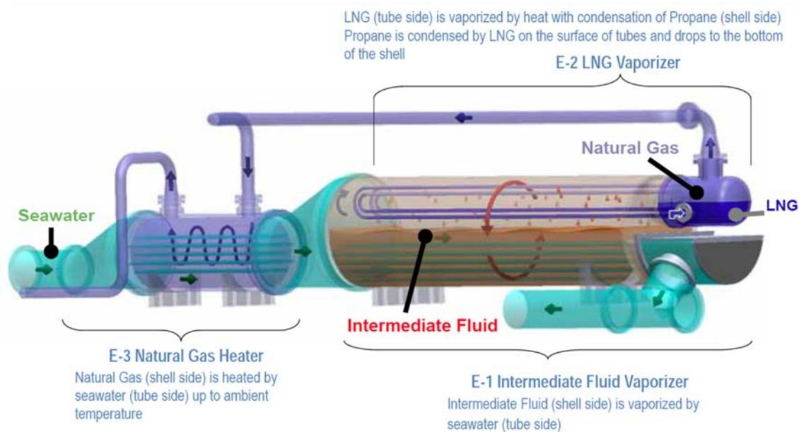
**Fig. 1 Intermediated Fluid type LNG vaporizer**
