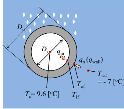
Fig. 2 Evaporation model on a single tube (Titanium)
