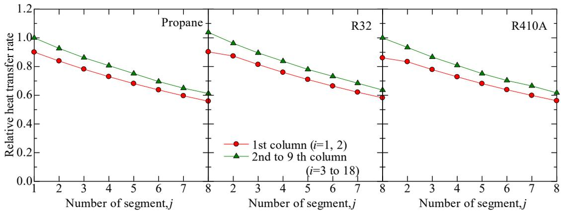
**Fig. 13 Heat transfer rate profile in evaporator tube bundles predicted by Eq. (8) (Ribatski et al., 2008) and NTU method.**
