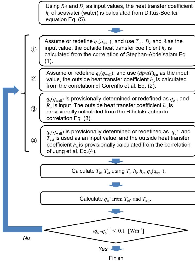
**Fig. 3 Evaporation calculation flow on a single tube**
