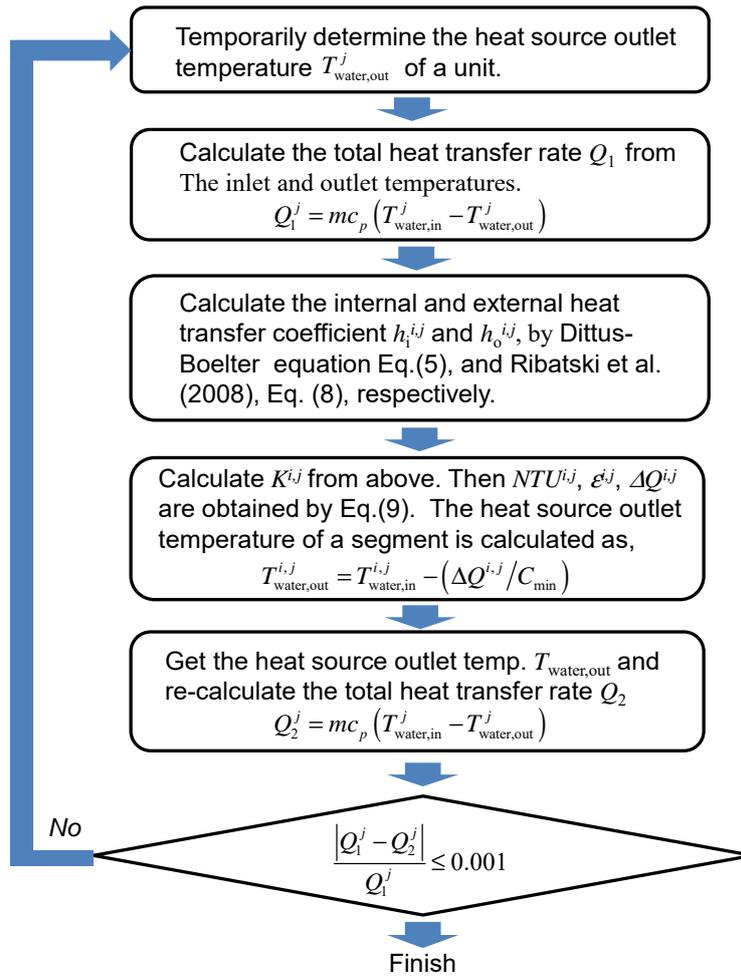
**Fig. 10 Calculation procedure for evaporator**
