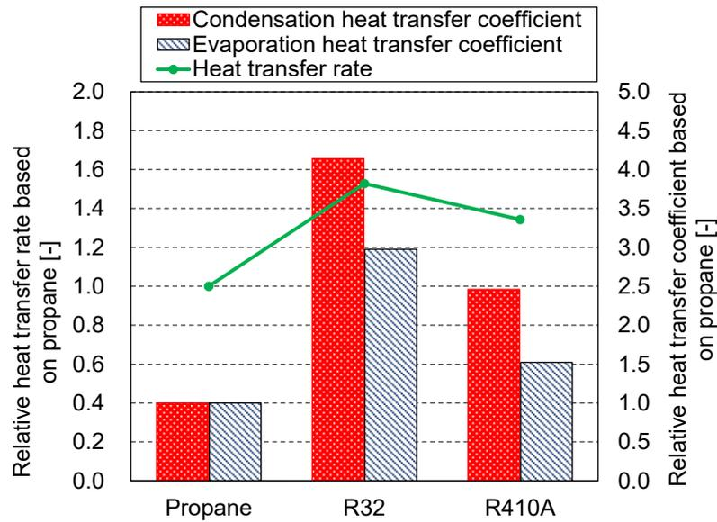
**Fig. 8 Experimentally determined heat transfer performance for the selected intermediate fluids.**
