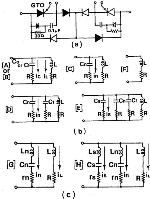
Fig 2. AC switch and filters.
