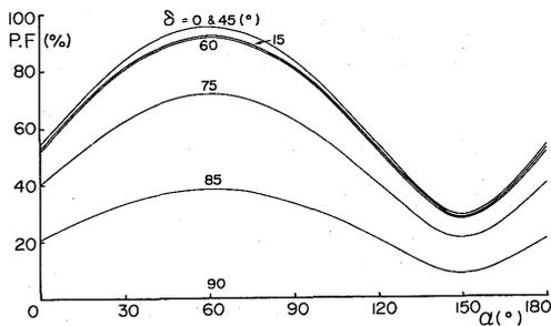
Fig 6. Input power factor P.F vers.  $\alpha$ . (RC filters type B)
