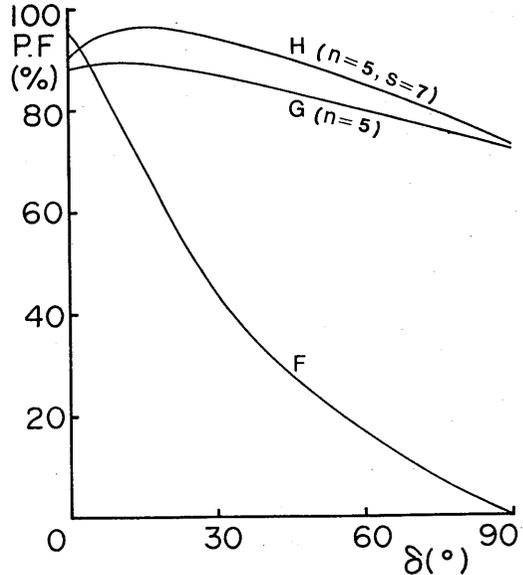
Fig 11. Input power factor P.F vers.  $\delta^\circ$ . (LC filters)
