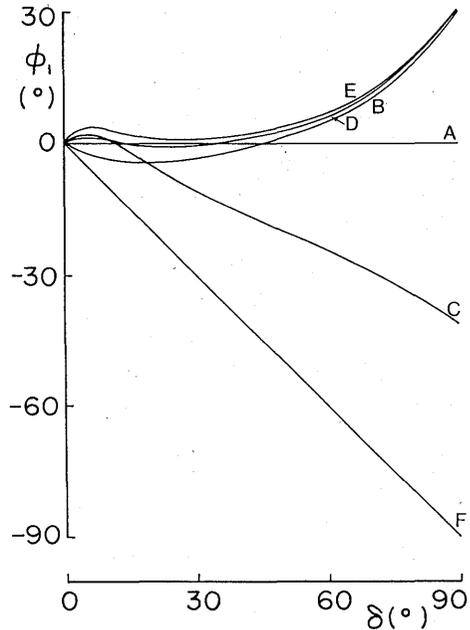
Fig 7. Fundamental displacement angle  $\phi_1$  vers. load angle  $\delta$ . (RC filters)
