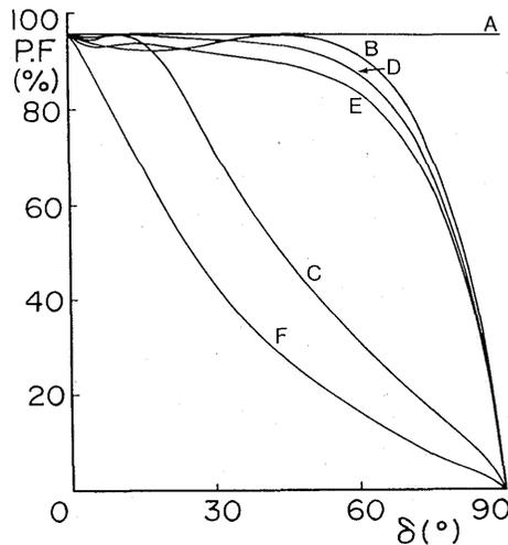
Fig 8. Input power factor P.F vers.  $\delta$ . (RC filters)
