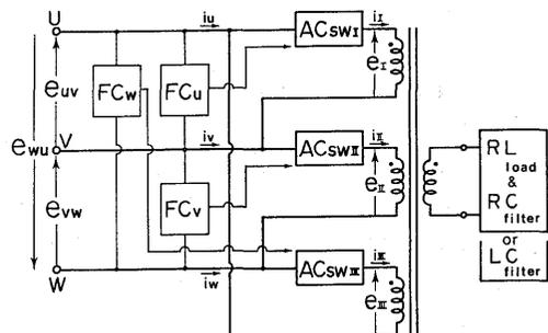
Fig 1. Main circuit of 3f changer.
