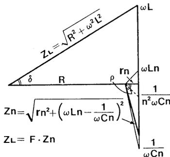
Fig 10. Vector diagram of LC filters Impedance  $Z_n$  and RL load Impedance  $Z_L$ .
