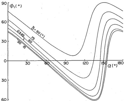
Fig 5. Fundamental displacement angle  $\phi_1$  vers. turn-on angle  $\alpha$ . (RC filters type B)
