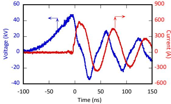
Figure 3. Voltage and current waveforms ( $\rho = 347 \text{ kg/m}^3$ ). The first peaks of voltage and current are determined as “breakdown voltage” and “arc current”, respectively.
