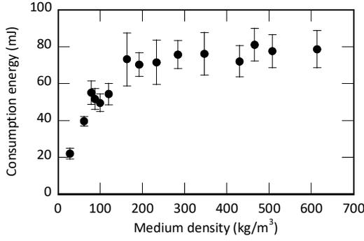
Figure 5. Consumption energy as a function of the medium density of CO<sub>2</sub>.
