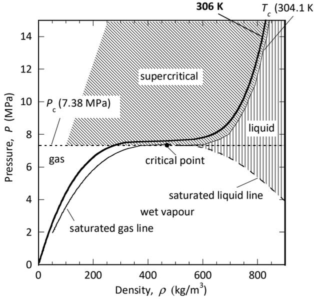
Figure 2. Phase diagram of carbon dioxide.
