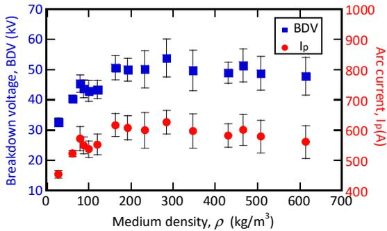
Figure 4. Pulsed breakdown voltage and pulse arc current as a function of the medium density of  $\text{CO}_2$
