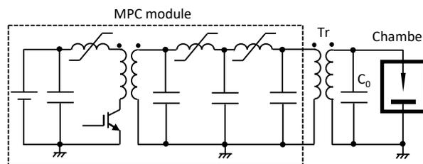
(b) Experimental circuit including MPC module
