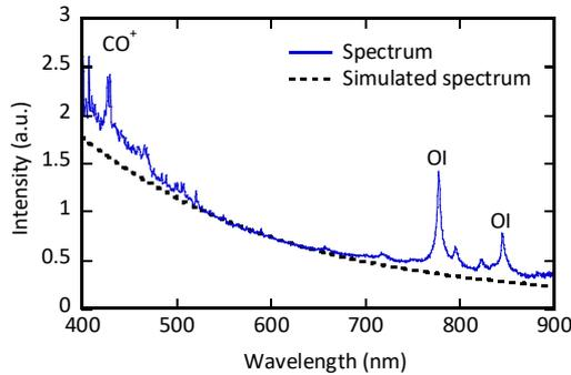
**Figure 8.** Optical emission spectra of pulsed arc discharge measured at ( $\rho = 347$  kg/m<sup>3</sup>) and simulated spectrum on the basis of a Planck's blackbody radiation law.
