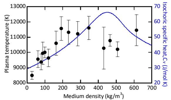
**Figure 9.** Plasma temperature and isochoric specific heat of CO<sub>2</sub> as a function of medium density of CO<sub>2</sub>.
