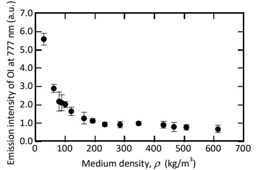
Figure 7. Variation of the emission intensity of OI (777 nm) as a function of the medium density of CO<sub>2</sub>.
