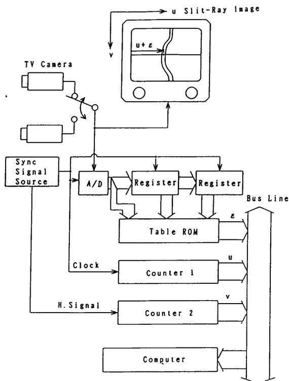
Fig. 2 Block diagram of image processor
