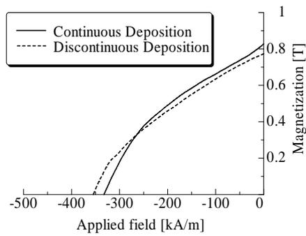
Fig.2 Demagnetization curves of crystallized multi-layered films prepared by continuous and discontinuous depositions.
