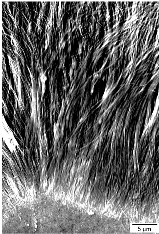
Fig. 4. SEM image of electrodeposited iron nanowires, which were separated from an AAO nanochannel template with the pore diameter of 33 nm.
