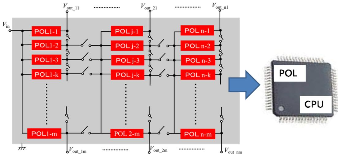
Fig. 4 Matrix-POL Power Supply System
