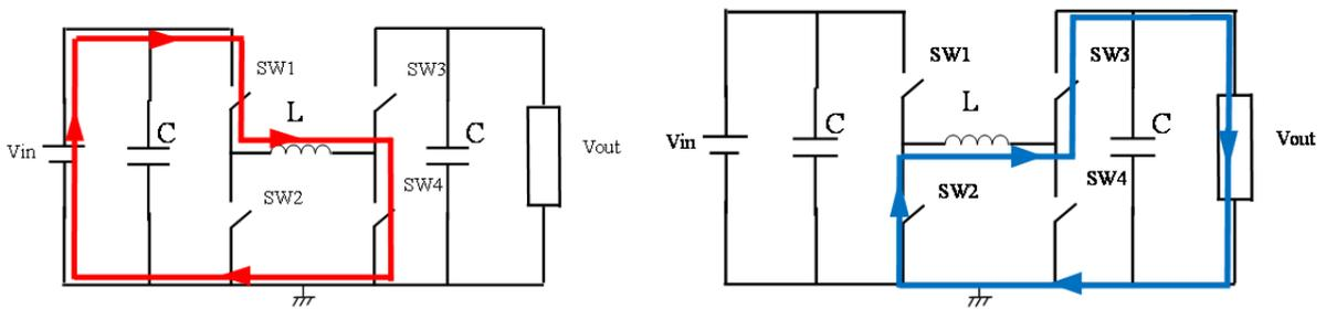
Fig. 6 H-bridge (Buck mode operation)
