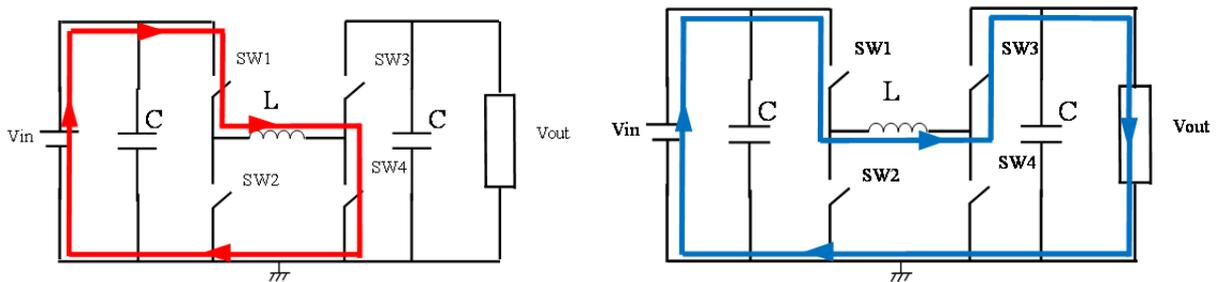
Fig. 7 H-bridge (Boost mode operation)
