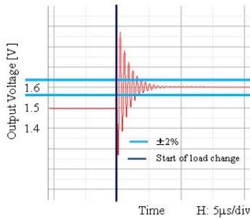
Fig. 13 Conventional off-chip POL
