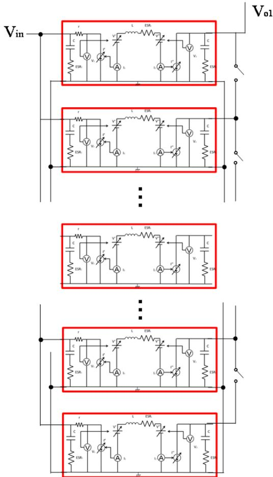
Fig. 10 Simulation circuit (Matrix-POL)
