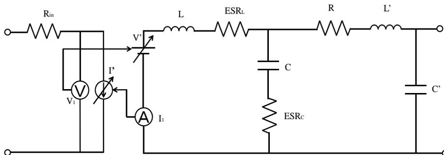
Fig. 9 Simulation circuit (Single POL)
