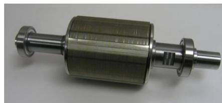
Fig. 10. Rotor with grain-oriented electric steel
