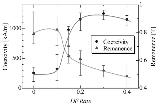
FIG. 2. Coercivity and remanence of films prepared from Nd<sub>2.6</sub>Fe<sub>14</sub>B target as a function of DF rate. The error bars indicate the maximum and the minimum values for 10–12 samples.
