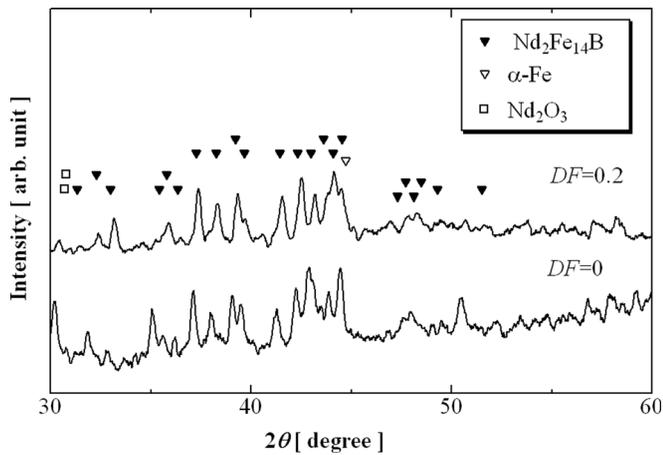
FIG. 1. X-ray diffraction patterns of crystallized film magnets.
