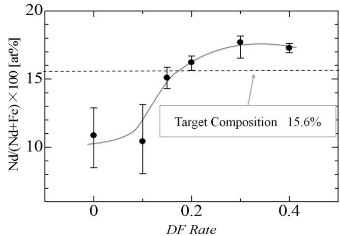
FIG. 3. Nd content in films prepared from Nd<sub>2.6</sub>Fe<sub>14</sub>B target as a function of DF rate. The error bars indicate the maximum and the minimum values for 10–12 samples.
