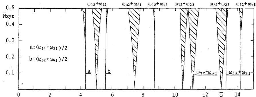
Fig. 8 Unstable regions of the rectangular plate: case I, type 2,  $\bar{N}_{xy0}=0.0$  and  $\mu=1.5$ .
