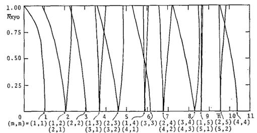
Fig. 4 Shearing force  $\bar{N}_{xy0}$  vs. natural frequency  $\bar{n}$ : case III and  $\mu = 1.0$ .
