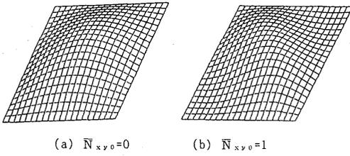
Fig. 5 Effect of shearing force  $\bar{N}_{xy0}$  on the modes of vibration: case I and  $\mu=1.0$ .
