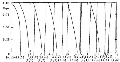
Fig. 3 Shearing force  $\bar{N}_{xy0}$  vs. natural frequency  $\bar{n}$ : case II and  $\mu = 1.0$ .
