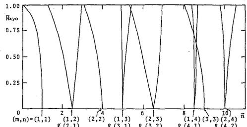
Fig. 2 Shearing force  $\bar{N}_{xy0}$  vs. natural frequency  $\bar{n}$ : case I and  $\mu = 1.0$ .
