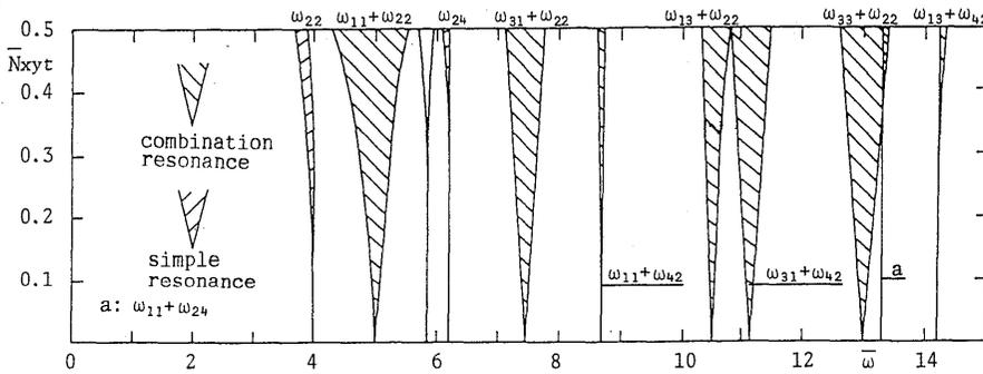
Fig. 7 Unstable regions of the rectangular plate: case I, type 1,  $\bar{N}_{xy0}=0.0$  and  $\mu=1.5$
