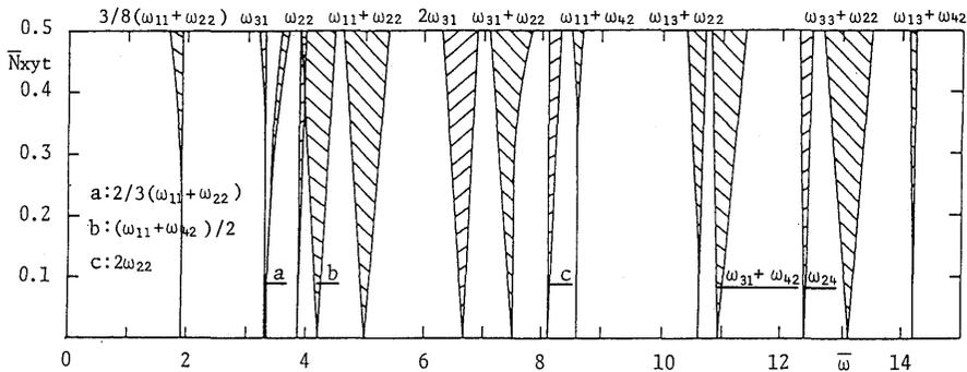
Fig. 13 Unstable regions of the rectangular plate: case I, type 1,  $\bar{N}_{xy0}=0.3$  and  $\mu=1.5$ .
