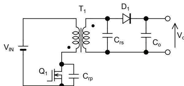
Fig.1 Circuit configuration of proposed converter
