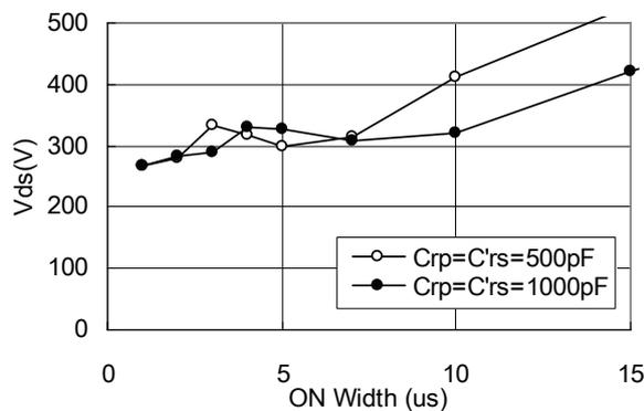
Fig.12 Simulated  $Q_1$  voltage in condition 5
