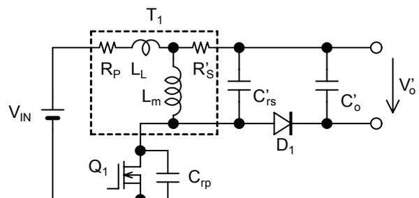
Fig.2 Equivalent circuit for analysis of operation
