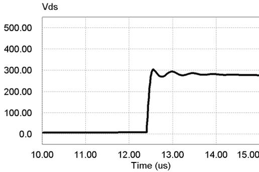
Fig.7 Simulated  $Q_1$  voltage waveform in condition 2 ( $C'_{rs}=1700pF$ )
