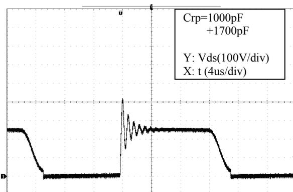
Fig.16 Vds waveform of conventional converter
