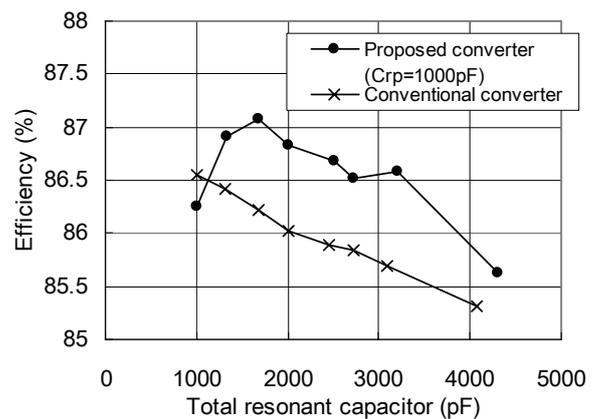
Fig.14 Measured efficiency of the prototype
