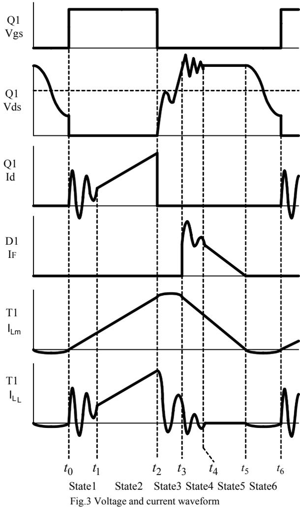
Fig.3 Voltage and current waveform
