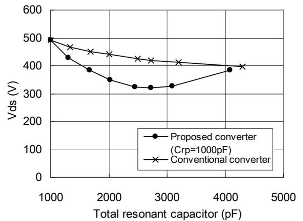
Fig.13 Measured  $V_{ds}$  voltage of the prototype
