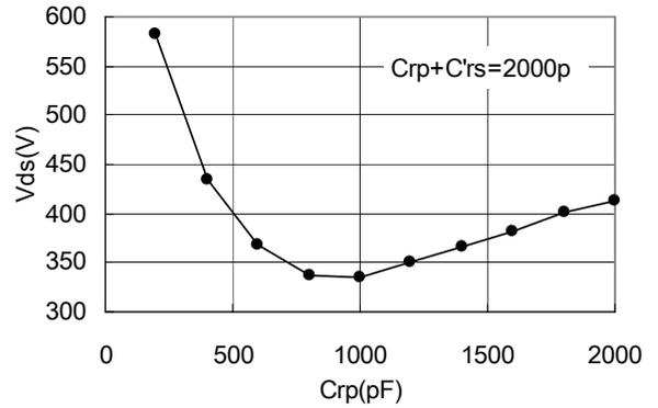
Fig.5 Simulated  $Q_1$  voltage in condition 1
