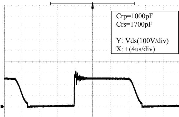
Fig.15 Vds waveform of proposed converter
