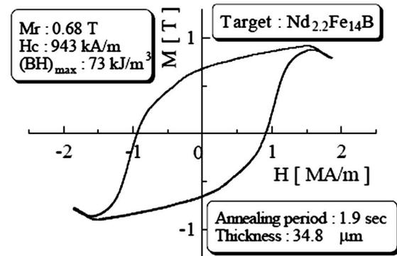
FIG. 5. An  $M$ - $H$  loop of PLD-made Nd–Fe–B thick film magnet by using a  $\text{Nd}_{2.2}\text{Fe}_{14}\text{B}$  target followed by pulse annealing for 1.9 s. The obtained remanence and  $(BH)_{\text{max}}$  values were larger than those prepared by using a  $\text{Nd}_{2.4}\text{Fe}_{14}\text{B}$  target.
