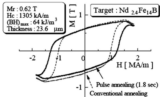
FIG. 3.  $M-H$  loops of PLD-made Nd-Fe-B thick film magnets crystallized by two methods of the pulse annealing and a conventional annealing process. These samples were prepared by using a  $Nd_{2.4}Fe_{14}B$  target. Coercivity of the film pulse annealed for 1.8 s was larger by approximately 300 kA/m compared with that annealed by a conventional method.
