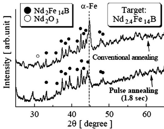
FIG. 4. X-ray diffraction patterns of PLD-made Nd–Fe–B thick film magnets after crystallization by two methods of the pulse annealing and a conventional annealing process. These samples were prepared by using a  $\text{Nd}_{2.4}\text{Fe}_{14}\text{B}$  target.
