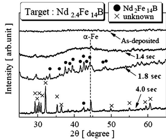
FIG. 2. X-ray diffraction patterns of PLD-made Nd-Fe-B thick film magnets prepared by a pulse annealing process under the various annealing period. These samples were prepared by using a  $Nd_{2.4}Fe_{14}B$  target.
