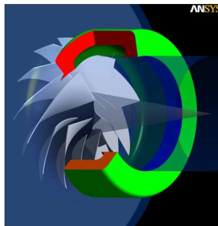
Fig.1 Centrifugal compressor with ring groove arrangement
