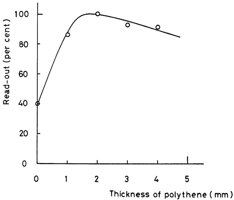
Fig. 2. Build up curve in 14-15 MeV neutron beam.
