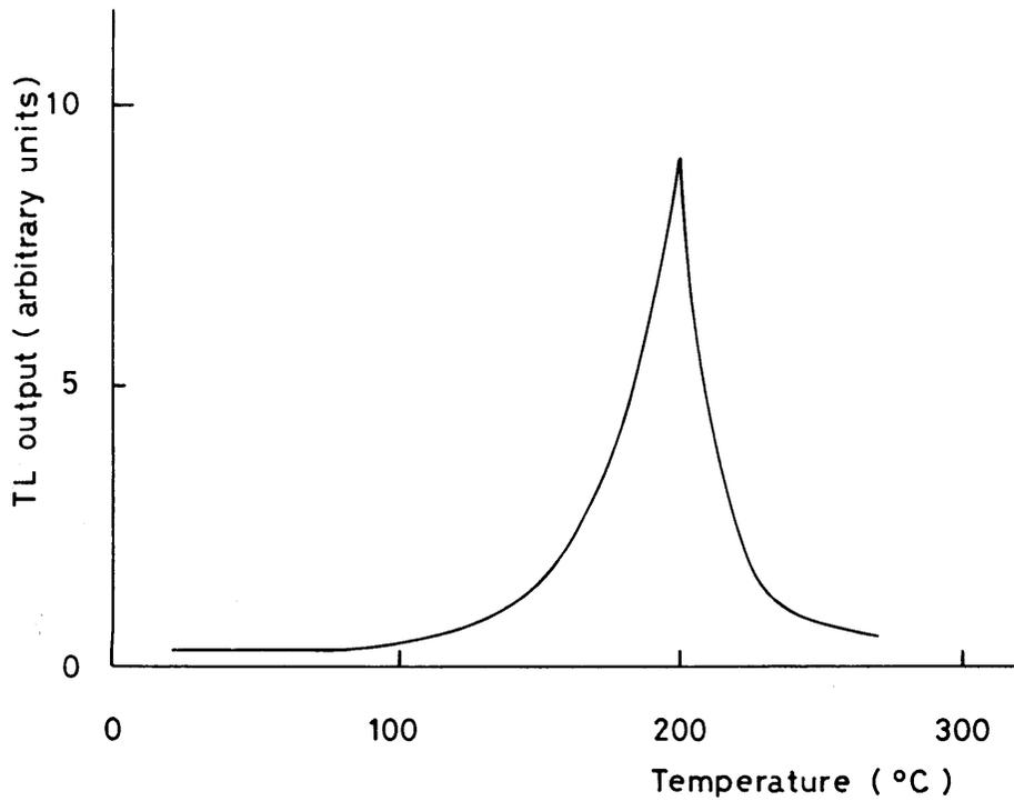
Fig. 1. Glow curve of MgB<sub>4</sub>O<sub>7</sub>: Tb phosphor measured at one day after irradiation.
