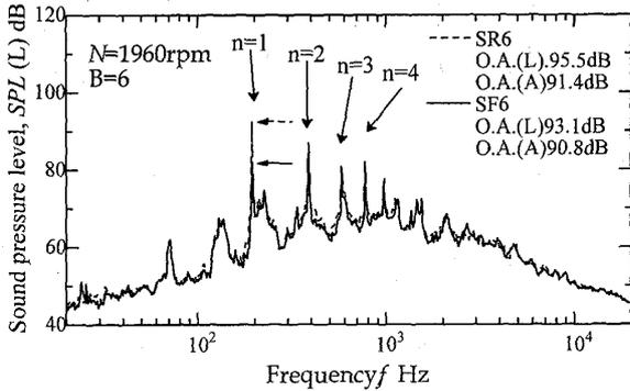
Fig.8 Spectral density distributions of the single-stage fan noise
