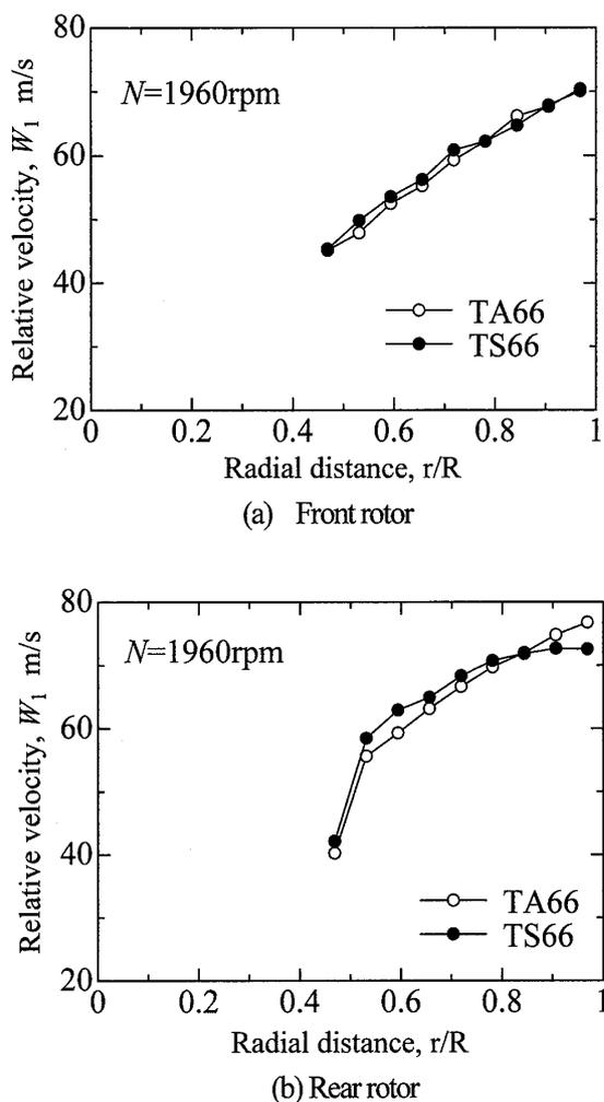
Fig.3 Radial distributions of the inlet relative velocity of the rotor
