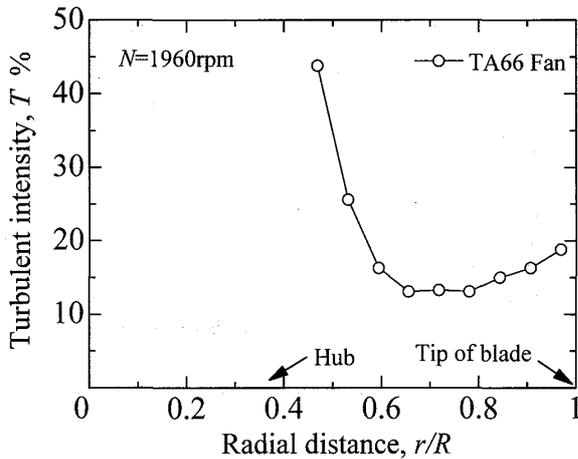
Fig.6 Radial distributions of the turbulent intensity
