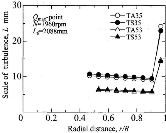
Fig.5 Radial distributions of the turbulent scale
