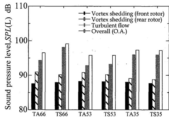
Fig. 9 Comparison of the two different sources
