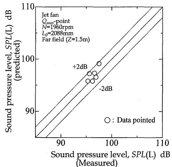
Fig.10 Comparison of predicted and measured sound pressure level of the turbulent noise
