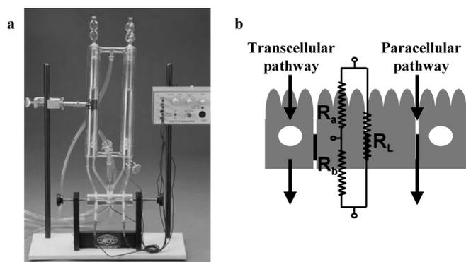
Fig. 1. (a) Ussing System Used in the Penetration Experiment and (b) Equivalent Circuit Model for Corneal Epithelium
