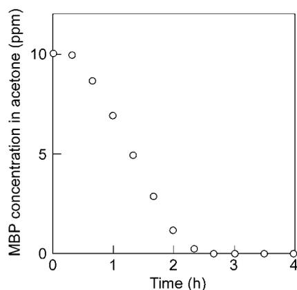
**Fig. 3.** Relationship between MBP Concentration in Acetone and Photolysis Period under Sunlight
