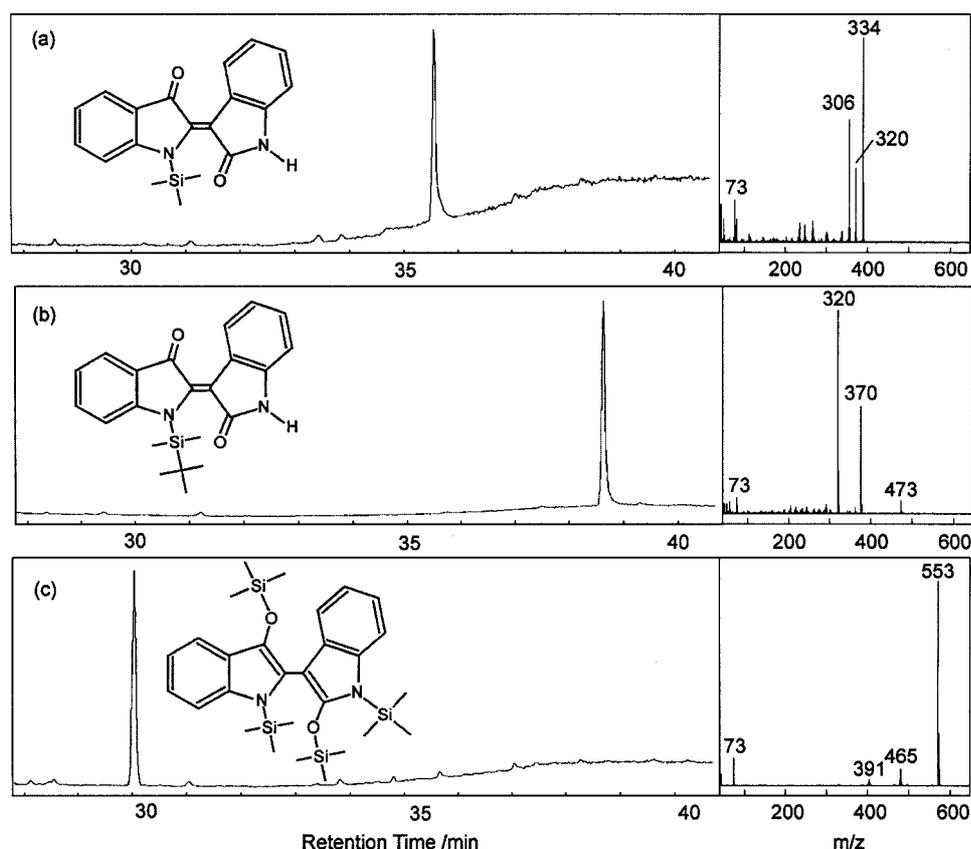
**Fig. 1.** Chromatograms, Structural Formulas and Mass Spectra of Indirubin after Reaction for 1 hr at 60°C
