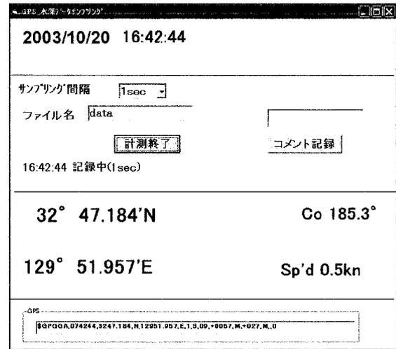
Fig. 4 An example screen of recording DGPS data. Date, time, position (latitude and longitude), speed and course are available to monitor.
