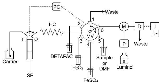
Fig. 1 SIA system for antioxidant assay of hydroxyl radical. SP, syringe pump, Cavro XL 3000 (syringe volume: 1 mL); HC, holding coil (length: 1 m, 0.5 mm, i.d.); MV, multi-port valve, Cavro Smart Valve; M, mixing tee; P, pump, Shimadzu LC-10ADvp; D, chemiluminescence detector, Shimadzu CLD-10A; I, integrator, Shimadzu Chromatopac C-R8A; PC, personal computer, NEC Alie NX; CL reagent solution, 200  $\mu\text{M}$  luminol solution.
