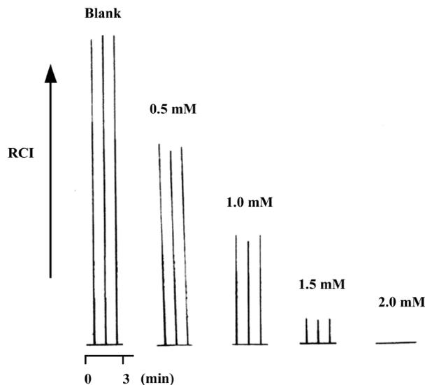
Fig. 3 Signal responses obtained for blank and L-ascorbic acid solutions. RCI: the CL intensity selected value was taken as 100. Carrier solution: 100 mM HEPES buffer (pH 7.4). Reagent solution: 200  $\mu$ M luminol solution (1% DMF) [flow rate, 1.0 mL/min], 2.5 mM H<sub>2</sub>O<sub>2</sub> in HEPES buffer (pH 7.4) [10  $\mu$ L], and 2.5 mM FeSO<sub>4</sub> in H<sub>2</sub>O [10  $\mu$ L]. Sample: DMF or L-ascorbic acid [5  $\mu$ L].
