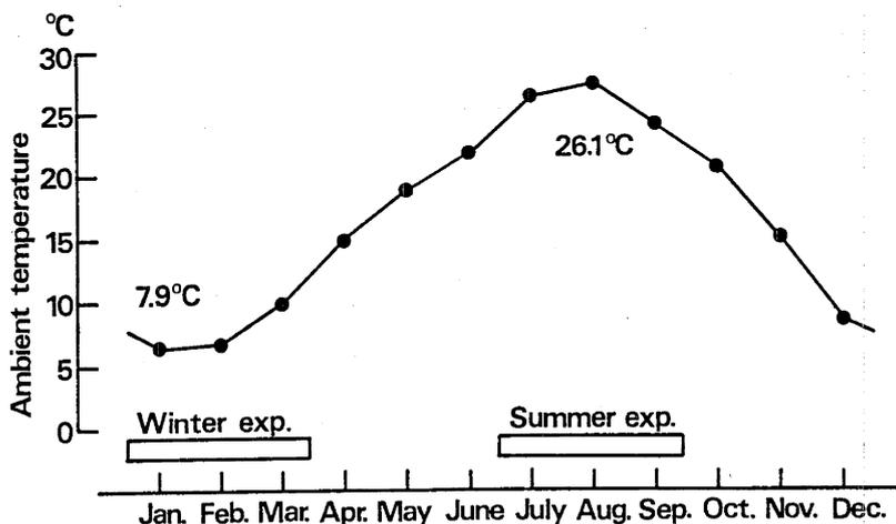
Fig. 1. Monthly mean ambient temperature in Nagasaki. Mean ambient temperature of the experimental period is 7.9°C in winter (January to March) and 26.1°C in summer (July to September).
