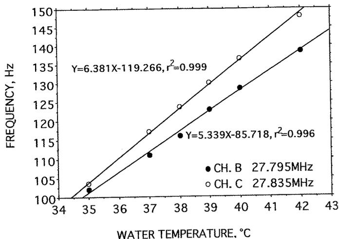
Fig. 1. Calibration of the transmitters. There was a linear correlation between water temperature and pulse frequency in the range between 35°C and 42°C in each transmitter.
