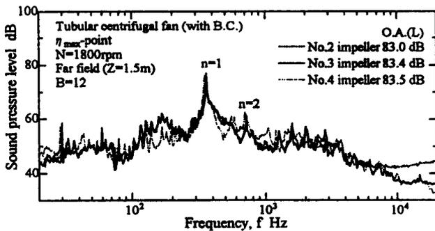
Fig. 7 Spectral distribution of fan noise. (With belt case)
