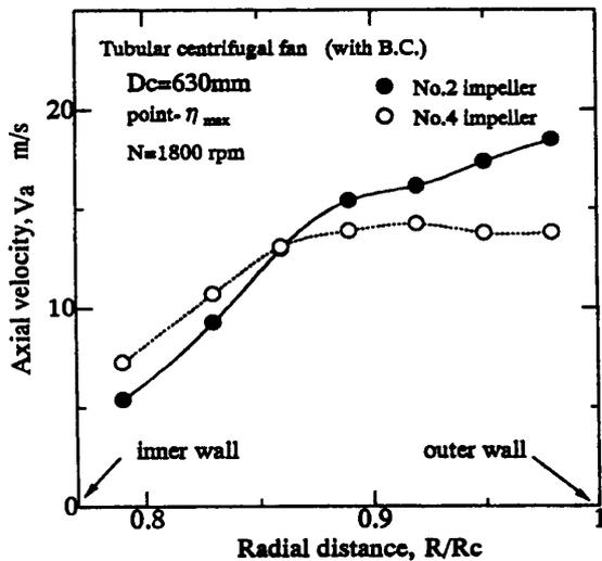
Fig. 6 Spanwise distributions of axial velocity. (Effects of inclination of the blade)
