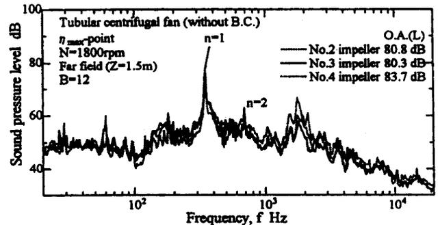
Fig. 8 Spectral distribution of fan noise. (Without belt case)
