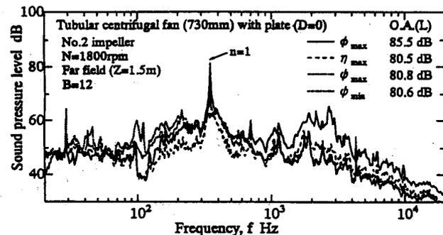
Fig.10 Spectral distribution of fan noise for each flow (Without belt case).
