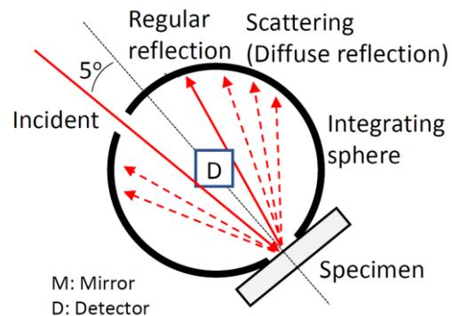
Fig. S2 Diffuse reflectance with integrating sphere.
