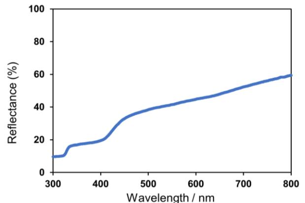
Fig. 2 UV-Vis reflectance spectrum of *T. labefactus* (pale-yellow, dead).
