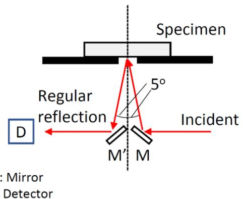
Fig. S1 Optical system of regular reflectance measurement.
