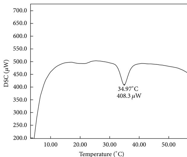
FIGURE 2: The typical DSC spectrum of the 1% concentration of TAC solution. Note that there are no peaks of  $T_g$  and  $T_c$ . The valley corresponding to  $T_m$  presents  $T_d$ .
