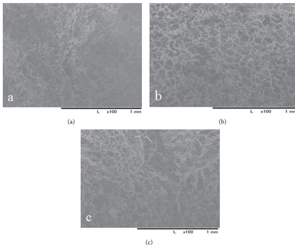
FIGURE 3: The surface images of sponges produced from different concentrations of TAC solution: (a) 0.5% (v/v), (b) 1.0% (v/v), and (c) 2.0% (v/v).
