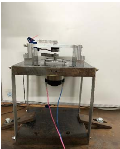
Fig.1 Experimental apparatus. (without displacement magnification mechanism)
