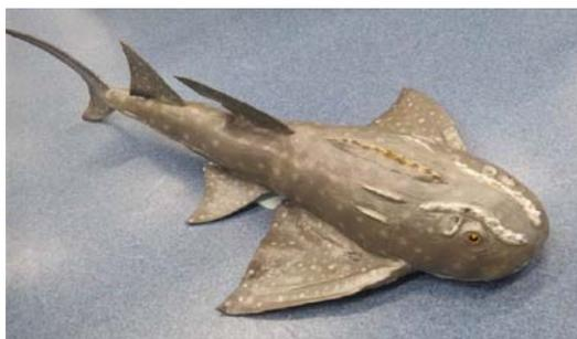
Fig. 1. Shark ray robotic fish.
