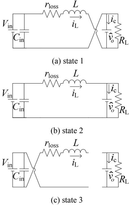
Figure 11. Equivalent circuit of boost mode operation: (a) state 1; (b) state 2; (c) state 3.
