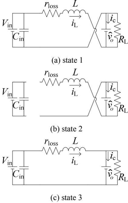
Figure 10. Equivalent circuit of buck mode operation: (a) state 1; (b) state 2; (c) state 3.
