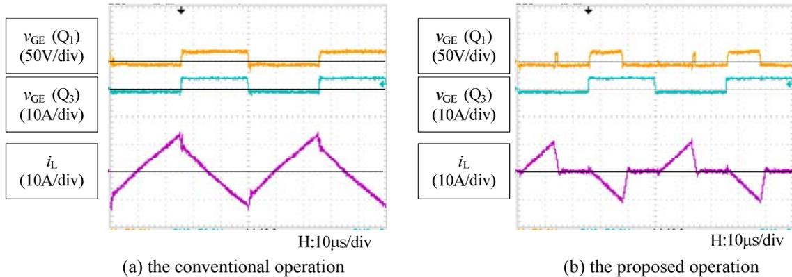
Figure 15. The comparison of the current waveforms of  $i_L$ : (a) the conventional operation ( $V_{\text{in}}=200\text{V}$ ,  $V_{\text{out}}=150\text{V}$ ,  $P_o=200\text{W}$ ); (b) the proposed operation ( $V_{\text{in}}=200\text{V}$ ,  $V_{\text{out}}=150\text{V}$ ,  $P_o=191\text{W}$ ).
