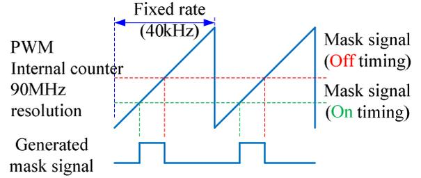
Figure 9. Mask signal generating mechanism by PWM peripheral in DSP.
