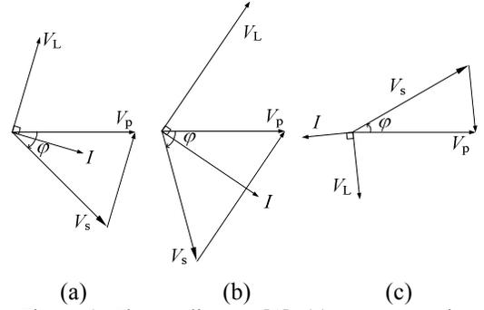
Figure 3. Phasor diagram[1]: (a) power running mode (light load); (b) power running mode (heavy load); (c) power regenerative mode.
