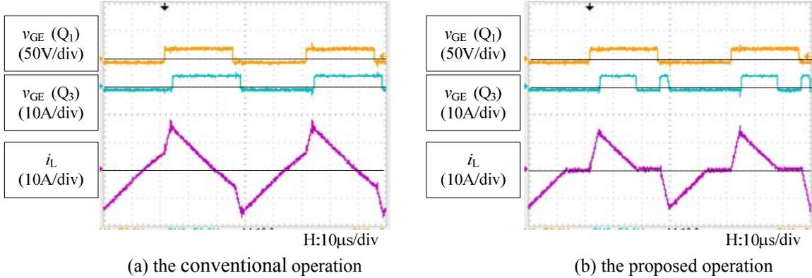
Figure 14. The comparison of the current waveforms of  $i_L$ : (a) the conventional operation ( $V_{\text{in}}=100\text{V}$ ,  $V_{\text{out}}=150\text{V}$ ,  $P_o=200\text{W}$ ); (b) the proposed operation ( $V_{\text{in}}=100\text{V}$ ,  $V_{\text{out}}=150\text{V}$ ,  $P_o=200\text{W}$ ).
