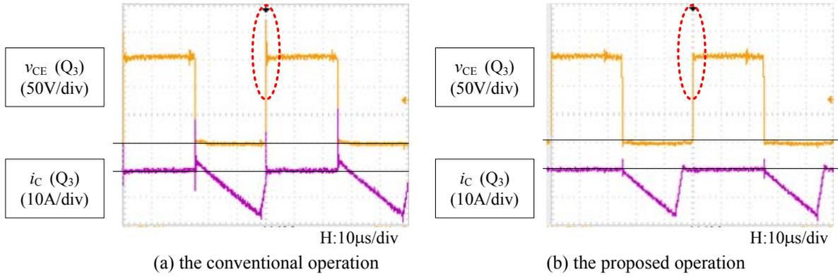
Figure 12. The waveforms in buck mode: (a) the conventional operation ( $V_{in}=200V$ ,  $V_{out}=150V$ ,  $P_o=504W$ ); (b) the proposed operation. ( $V_{in}=200V$ ,  $V_{out}=150V$ ,  $P_o=502W$ )
