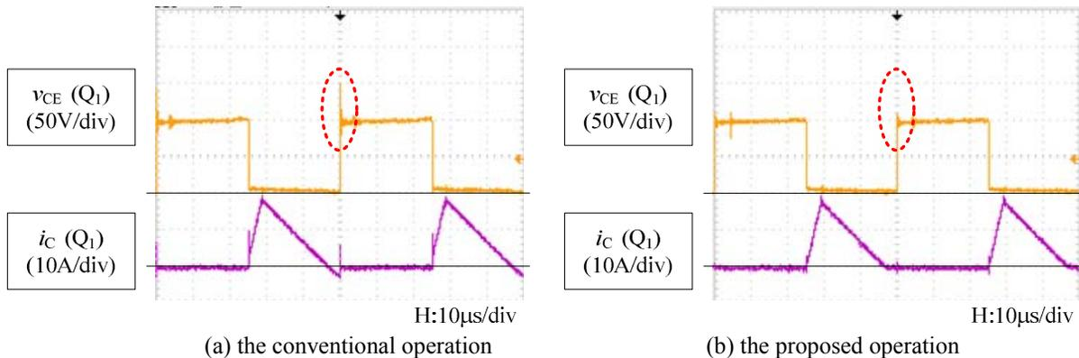
Figure 13. The waveforms in boost mode: (a) the conventional operation ( $V_{in}=100V$ ,  $V_{out}=150V$ ,  $P_o=687W$ ); (b) the proposed operation. ( $V_{in}=100V$ ,  $V_{out}=150V$ ,  $P_o=686W$ )
