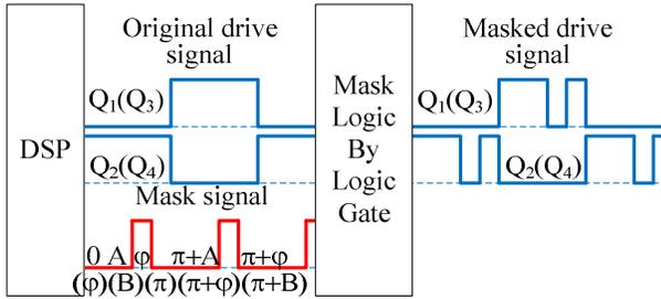
Figure 8. Masked drive signal generating mechanism.
