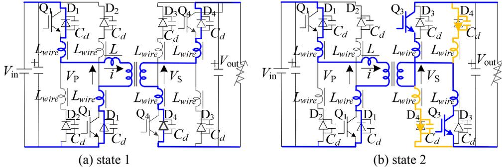
Figure 5. The generation mechanism of switching surge.
