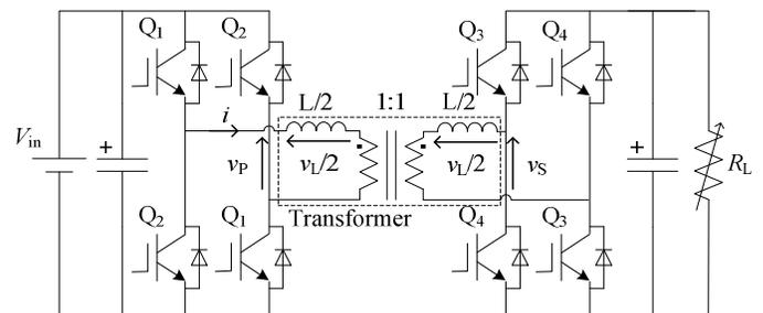
Figure 1. The circuit schematic of DAB dc-dc converter.
