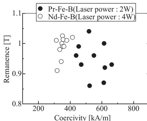
FIG. 3. Coercivity and remanence values of annealed Pr-Fe-B and Nd-Fe-B/ $\alpha$ -Fe thick-films. The Pr-Fe-B films were prepared by using the laser energy density at approximately  $50 \text{ mJ/m}^2$  using the laser power of 2 W. The plots of Nd-Fe-B ones were also shown in Fig. 1. The remanence values of Pr-Fe-B thick-films fluctuated between 0.85 and 1.05 T, however the values of coercivity were higher compared with those of Nd-Fe-B/ $\alpha$ -Fe thick-films.
