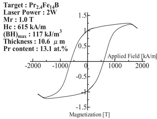
FIG. 4. In-plane M-H loop of an annealed Pr-Fe-B film which had the largest  $(BH)_{\max}$  value in the experiment. The film was prepared by using the laser energy density at approximately  $50 \text{ mJ/mm}^2$  using the laser power of 2 W. (Pr<sub>2.4</sub>Fe<sub>14</sub>B target).
