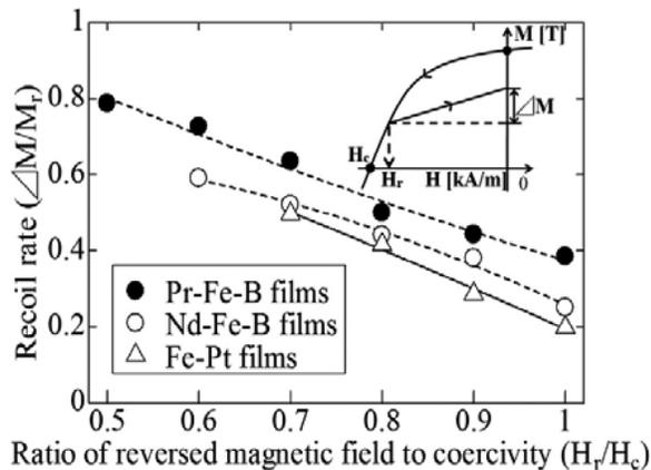
FIG. 5. Recoil rates of Pr-Fe-B, Nd-Fe-B/ $\alpha$ -Fe nano-composite, and Fe-Pt thick-films prepared by using the PLD method. As shown in the inset figure, the horizontal and vertical axes showed a ratio of reversed magnetic field to coercivity and a recoil rate, respectively.
