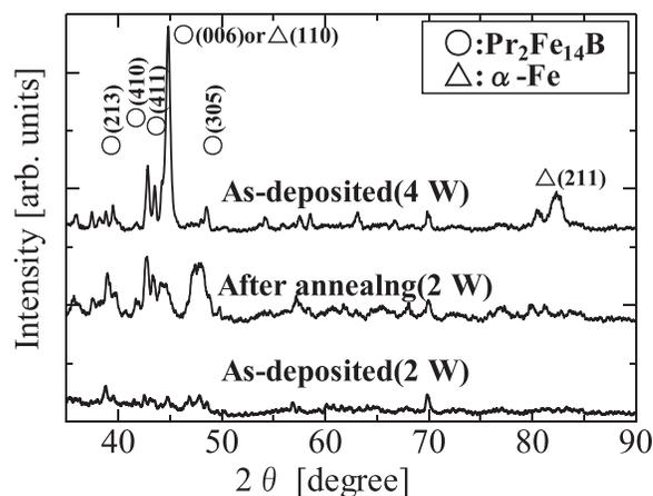
FIG. 2. X-ray diffraction patterns of as-deposited and annealed Pr-Fe-B films prepared by using a  $\text{Pr}_{2.4}\text{Fe}_{14}\text{B}$  target together with the laser power of 2 W. XRD pattern of an as-deposited film prepared at 4 W was also shown.
