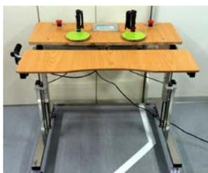
Fig.1 The effective wrist rehabilitation robot
