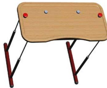
Fig.6 The CAD design of the new rehabilitative training robot for hospital use
