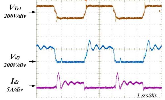
Fig.7. Experimental waveforms of surge occurrence (with snubber capacitance  $C_s=5\text{nF}$ )
