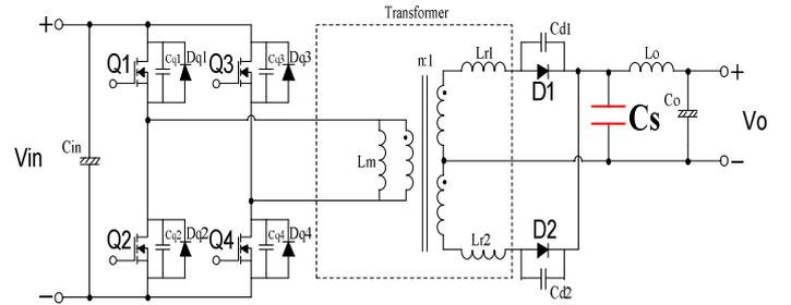
Fig.5. Full-bridge isolated DC-DC converter with Snubber Capacitor  $C_s$
