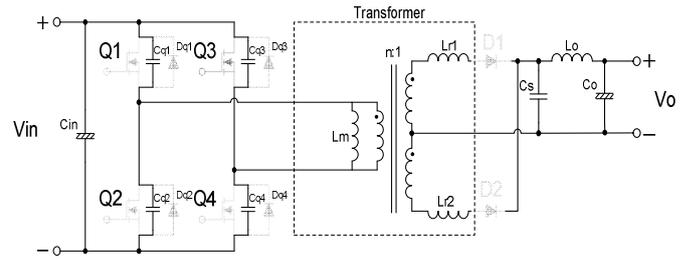
Fig.8. Circuit state during the dead time
