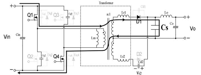
Fig.9. Surge current paths at turn-on time of primary switches
