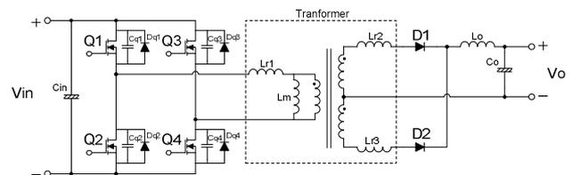
Fig.2. Circuit topology of full-bridge isolated DC-DC converter
