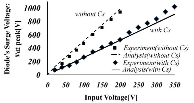
Fig.12. Analytical and experimental results for diode's surge voltage (Cs=50nF, Io=2A, Cd1=Cd2=200pF, Lr1=Lr2=Lr=2μH)
