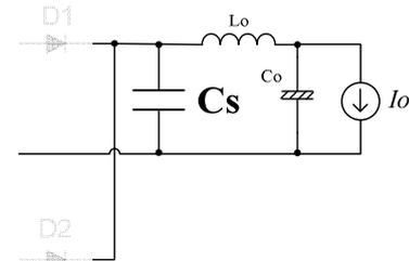
Fig.11. Equivalent circuit during the dead time
