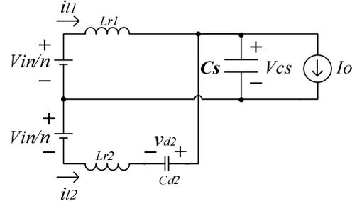
Fig.10. Equivalent circuit for surge current path at turn-on time of primary switches
