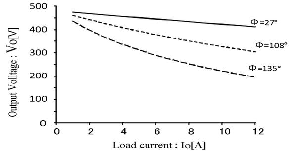
Fig. 16. Control characteristics of the converter with snubber capacitor  $C_s$ .
