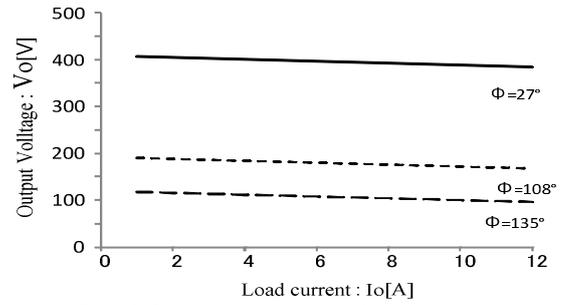
Fig. 15. Control characteristics of the converter without snubber capacitor  $C_s$ .
