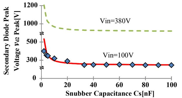
Fig.13. Effect of snubber capacitance on diode's surge voltage. (Comparison of analysis and experiment: Vin=100V, Io=2A, Cd1=Cd2=200pF, Lr=2μH)
