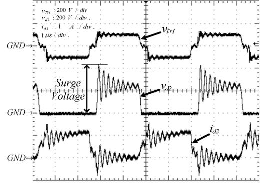
Fig.3. Experimental waveform of surge occurrence.
