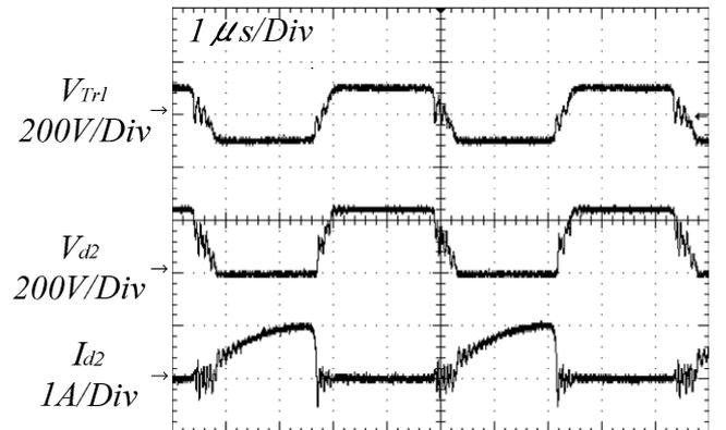
Fig.6. Experimental waveforms of surge occurrence (with snubber capacitance  $C_s=1.1\mu\text{F}$ ).
