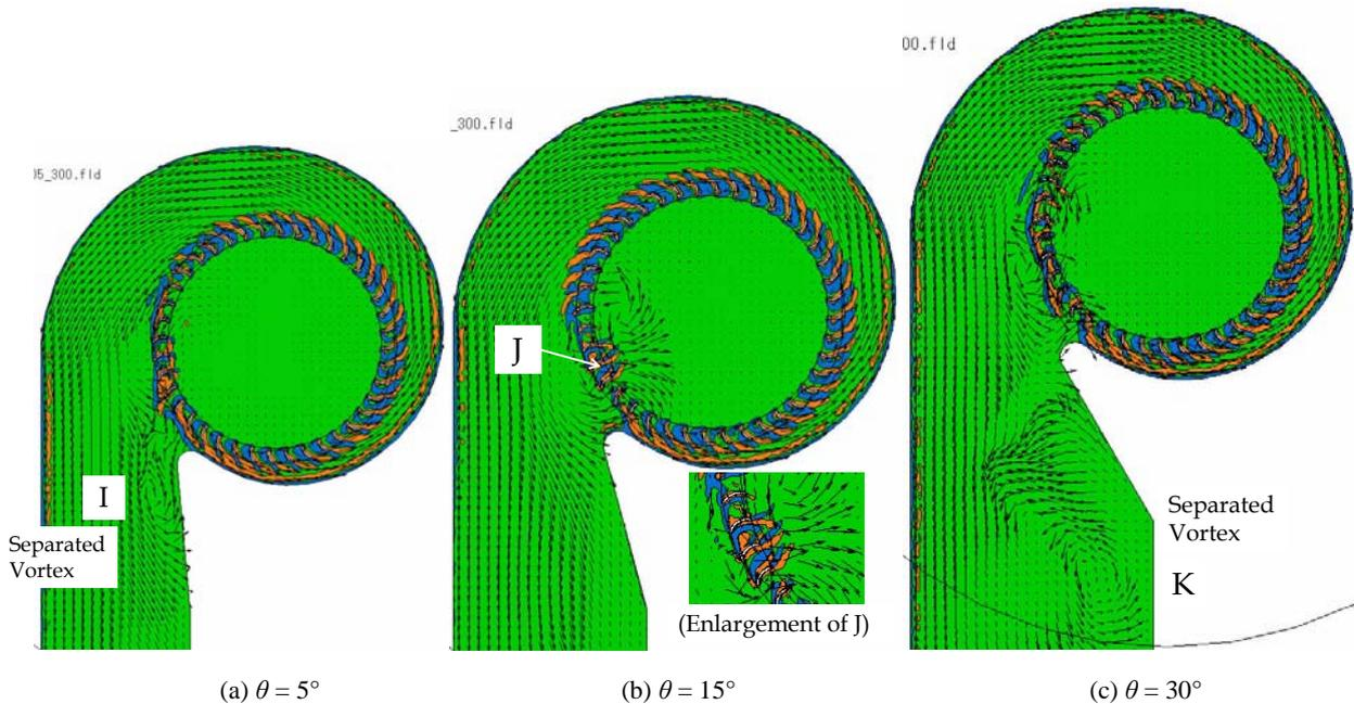
Fig. 13 Distribution of the aerodynamic noise sources and the velocity vectors for different outlet angles
