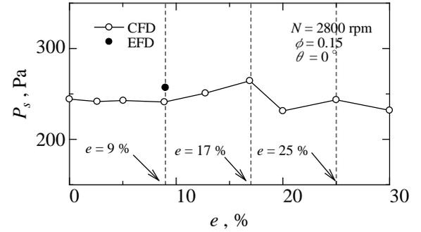
Fig. 7 Static pressure with respect to the bare ratio
