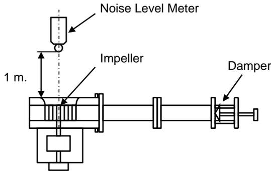
Fig. 3 Method of measuring the fan noise
