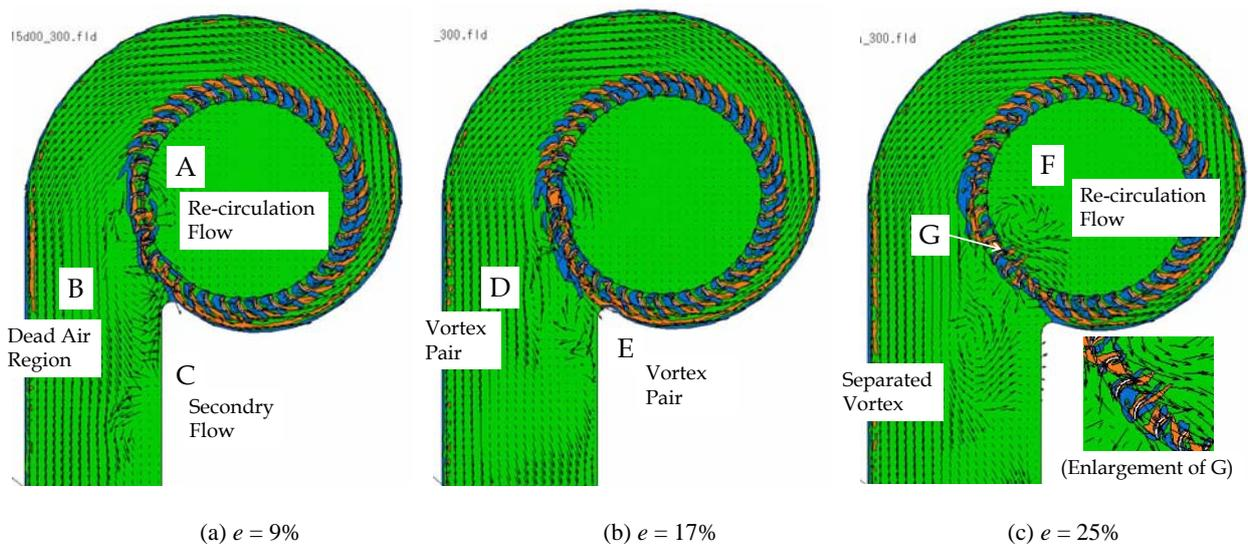
Fig. 10 Distribution of the aerodynamic noise sources and the velocity vectors for different base ratios
