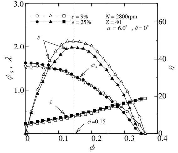
Fig. 6 Comparison of the aerodynamic characteristics for different bare ratios
