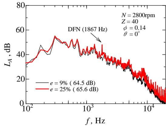
Fig. 9 Spectral distribution of the fan noise for different bare ratios
