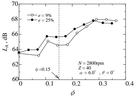
Fig. 8 Comparison of the fan noise for different bare ratios
