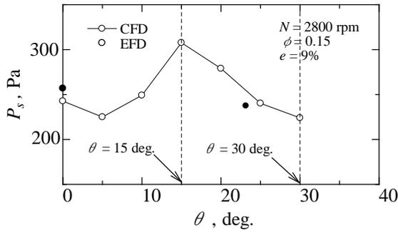
Fig. 11 Static pressure with respect to the outlet angle
