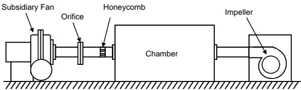
Fig. 2 Method for measuring the aerodynamic characteristics
