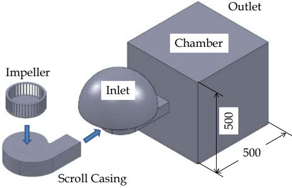
Fig. 5 Model for the numerical simulation
