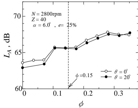
Fig. 12 Comparison of the fan noise characteristics for different outlet angles
