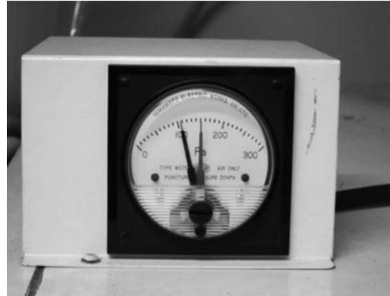
Fig. 9. Manometer of intermediate filter
