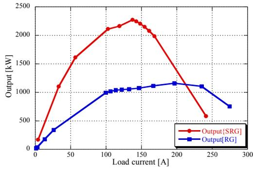
Figure 7. Output characteristics
