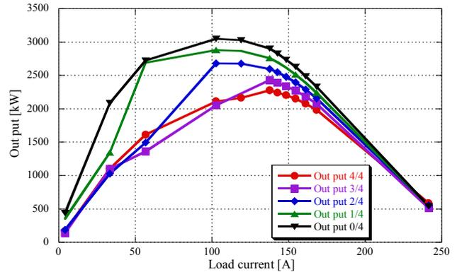
Figure 10. Output characteristics
