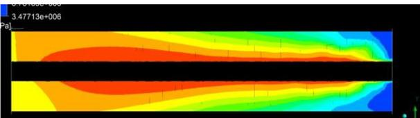
Figure 6. Osmotic pressure diagram of a hollow fiber area
