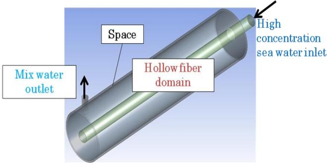
Figure 2. Symuration model of module
