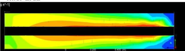
Figure 7. Amount of osmosis diagram of a hollow fiber area
