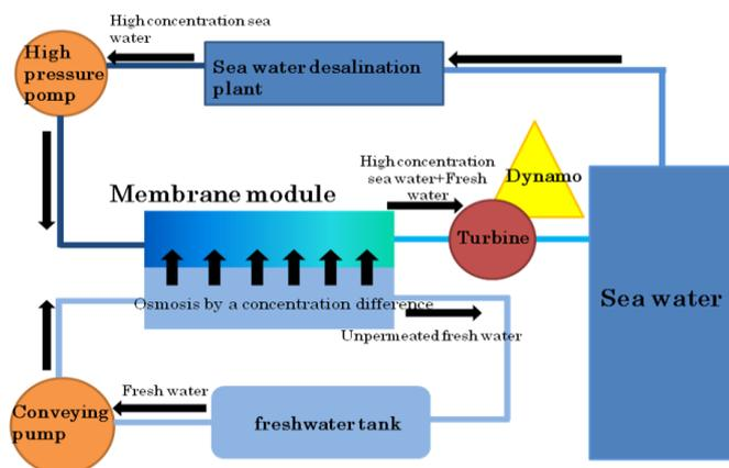
Figure 1. Whole figure of Power Generation
