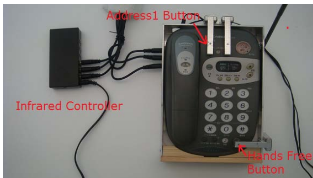
Fig 11. Telephone controlled with infrared signal
