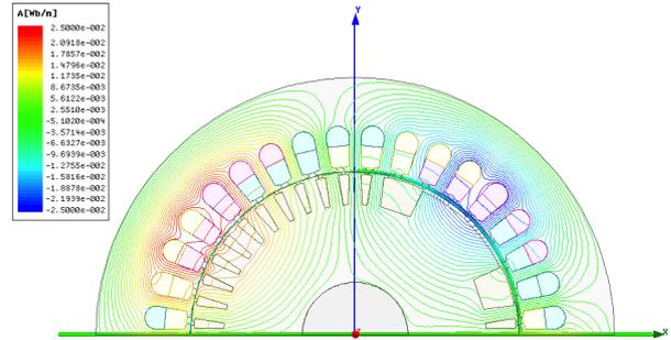
(c) Magnetic flux distribution produced by armature current at  $\omega t=0^\circ$ .
