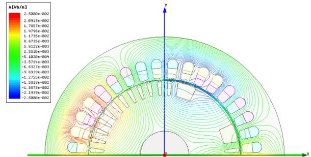
(d) Magnetic flux distribution produced by armature current at  $\omega t=60^\circ$ .
