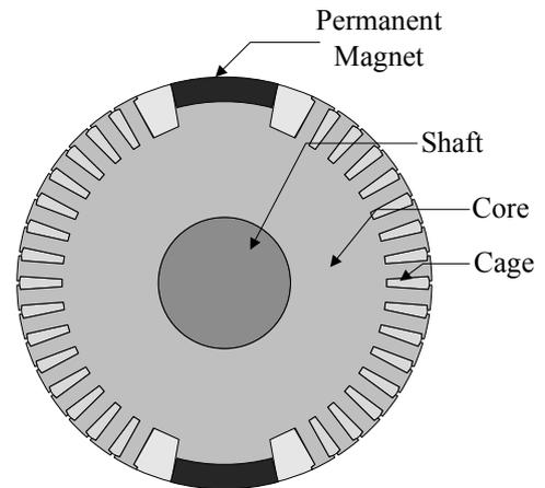
Fig. 2. Proposed rotor configuration.
