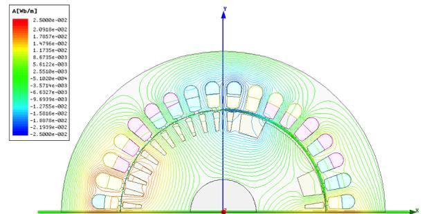
(e) Magnetic flux distribution produced by armature current at  $\omega t=120^\circ$ .
