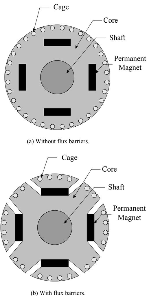
Fig. 1. Basic rotor configurations.
