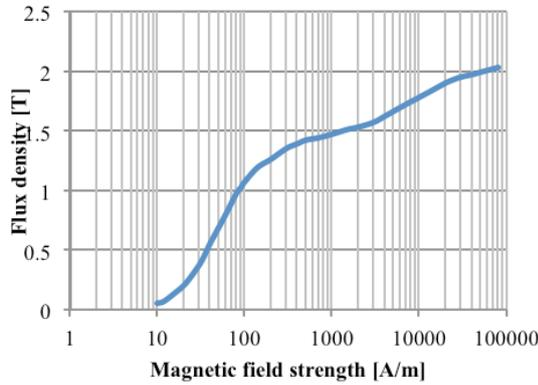
Fig. 4. B-H curve of the core material (50H250).
