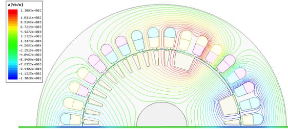
(b) Magnetic flux distribution produced by magnets.
