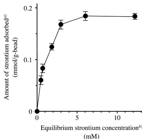
Fig. 1. Adsorption Isotherm of Strontium to PGMA-EGDMA-TTA-MP Beads
