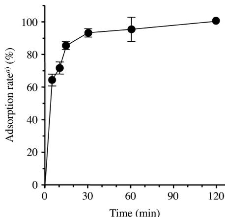
Fig. 2. Time-Course of Adsorption of Strontium to PGMA-EGDMA-TTA-MP Beads
