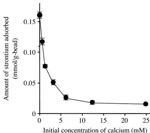
Fig. 3. Adsorption of Strontium to PGMA-EGDMA-TTA-MP Beads in the Presence of Increasing Calcium Ion Concentration
