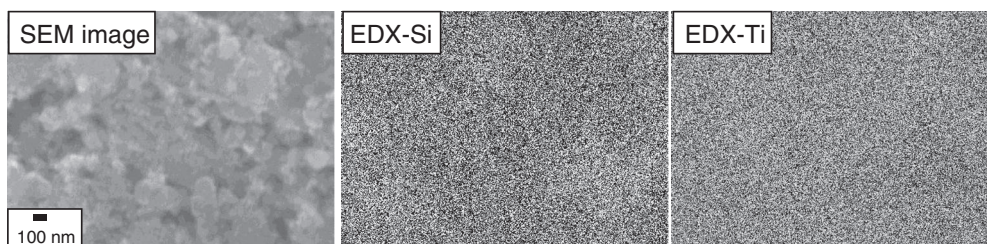
Figure 1. FE-SEM and EDX images of the nanocomposite of LSO-TO with a volume fraction of \text{TiO}_2 of 0.4.
