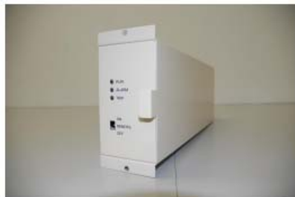
Fig.7. External view of a prototype SiC-SIT circuit breaker.
