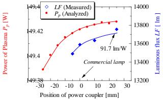
Fig. 6 Dependences of  $P_p$  and measured luminous flux LF on the position of the power coupler.
