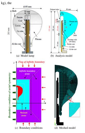
Fig.1 Analysis objects and model. A spherical electrodeless discharge lamp (150W type) with inner coil produced by Panasonic Electric Works, Ltd. was used as based model in this study.
