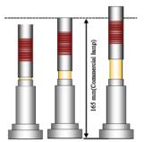
Fig.4 Schematic representation of change in the top position of the ferrite core.
