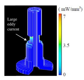
Fig. 5 Eddy current per unit volume in the power coupler.
