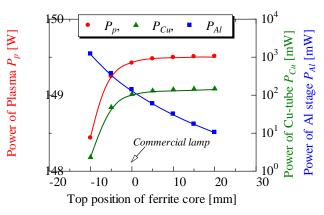
Fig. 3 Dependences of transmitted power to plasma  $P_p$ , consumed powers in Cu-tube  $P_{Cu}$  and Al stage  $P_{Al}$  on the top position of the ferrite core. The position for a commercial lamp is 165 mm.
