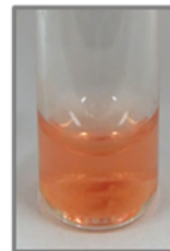
Fig. 3 Formation of glutathione selenotrisulfide by Painter reaction and its degradation to the red elemental selenium in phosphate buffer (pH 7.4).
