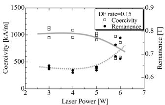
FIG. 4. Coercivity and remanence as a function of laser power. DF rate was set to 0.15.
