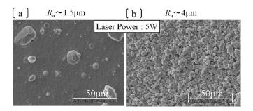
FIG. 7. SEM images of the film surface prepared using DF rate = (a) 0 and (b) 0.3. The average surface roughness is also shown.
