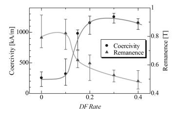
FIG. 2. Coercivity and remanence of films prepared from  $Nd_{2.6}Fe_{14}B$  target as a function of DF rate. The error bars indicate the maximum and the minimum values for 10–12 samples.
