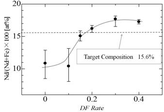
FIG. 3. Nd content in films prepared from  $Nd_{2.6}Fe_{14}B$  target as a function of DF rate. The error bars indicate the maximum and the minimum values for 10–12 samples.
