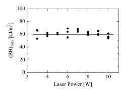
Fig. 7.  $(BH)_{\rm max}$  as a function of laser power. In the wide range of laser power between 3 and 10 W, the  $(BH)_{\rm max}$  showed the constant value of approximately 60 kJ/m<sup>3</sup>.
