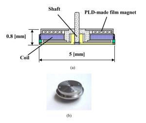
Fig. 10. Structure of a dc brush-less motor comprising a  $200-\mu$  m-thick PLD-made Nd–Fe–B film magnet. It rotates at 15160 rpm under no-load test, and has torque constant of 0.0236 mNm/A. (a) Schematic diagram of a milli-size motor. (b) Photograph of a milli-size motor.
