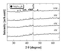
Fig. 5. X-ray diffraction patterns of annealed Nd–Fe–B thick film magnets. The films were prepared under various laser powers. The peaks corresponding to  $Nd_2Fe_{14}B$  phases were observed in all the samples.
