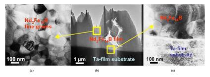
Fig. 8. Photos of TEM observations and cross sectional view for an isotropic Nd–Fe–B film magnet. (a) inside a sample, (b) TEM image in low magnification, (c) boundary on a Ta substrate.
