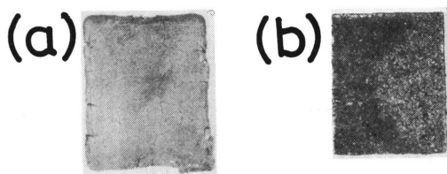
Photo. 3 Surface appearances of the sample oxidized at 1173 K. ( \times 0.8 ) (a) plain copper after 30h (b) aluminium diffusion coated copper (993 K, 7.5 h) after 109 h
