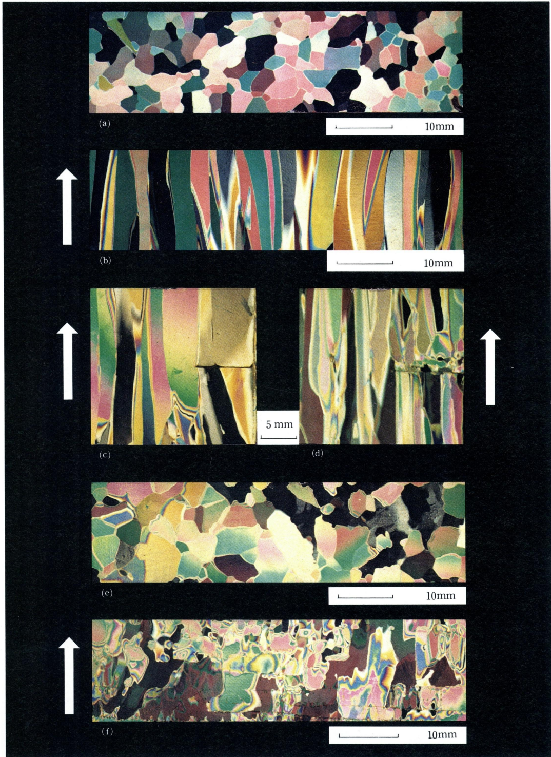
(a) Horizontally sliced (C. G. I. \alpha = 0^\circ ) (d) Central part of Seeding II (C. G. I. \alpha = 90^\circ ) (b) Vertically sliced (C. G. I. \alpha = 0^\circ ) (e) Horizontally sliced (Lam. I.) (c) Central part of Seeding I (C. G. I. \alpha = 90^\circ ) (f) Vertically sliced (Lam. I.)
