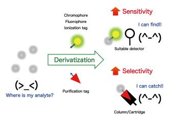
Derivatization technique can improve the detection sensitivity and control the chromatographic/extraction selectivity.
