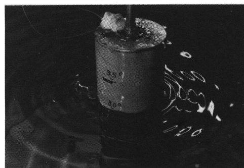
Photo. 4 Wave form at input acceleration level 9.8 gal
