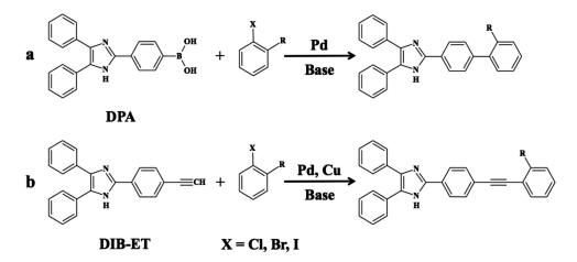
Fig. 1 Fluorescence derivatization of aryl halide by (a) the reaction with DPA based on the Suzuki coupling reaction and (b) the reaction with DIB-ET based on the Sonogashira coupling reaction (proposed method).
