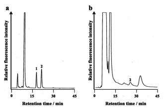
Fig. 6 Chromatograms of bromoanisole derivatives obtained by (a) the reaction with DIB-ET and (b) the reaction with DPA. Peaks: 1, o-bromoanisole derivative; 2, p-bromoanisole derivative. Sample concentration: 50  $\mu$ M for all compounds.
