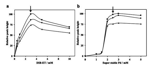
Fig. 2 Effect of the reagent concentrations and reaction conditions on the peak heights of aryl bromides. Where (a) effect of DIB-ET concentration, (b) effect of super stable Pd concentration. Compounds:  $\blacksquare$ , *p*-bromoanisole;  $\bullet$ , bromobenzene;  $\blacktriangle$ , *p*-bromotoluene and sample concentration: 50  $\mu$ M for all compounds.
