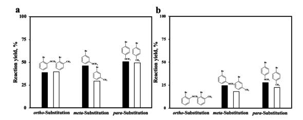
Fig. 5 Reactivities of (a) DIB-ET and (b) DPA to *ortho-*, *meta-*, *para-*substituted bromobenzenes. Sample concentration:  $50 \,\mu$ M for all compounds.
