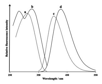
Fig. 3 Fluorescence spectra of the  $0.5 \,\mu\text{M}$  DIB-ET and  $0.5 \,\mu\text{M}$  bromobenzene derivative with DIB-ET. Excitation spectra of (a, dashed line) DIB-ET with emission at 400 nm and (b, solid line) bromobenzene derivative with emission at 430 nm. Emission spectra of (c, dashed line) DIB-ET with excitation at 310 nm and (d, solid line) bromobenzene derivative with excitation at 330 nm.
