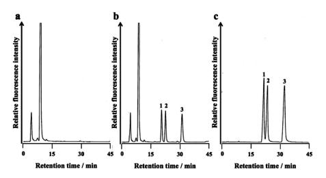
Fig. 4 Chromatograms of (a) reagent blank, (b) reaction mixture and (c) synthesized aryl bromide derivatives. Peaks: 1, *p*-bromoanisole derivative; 2, bromobenzene derivative; 3, *p*-bromotoluene derivative. Sample concentration:  $50 \,\mu$ M for all compounds.
