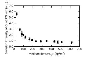
Figure 7. Variation of the emission intensity of OI (777 nm) as a function of the medium density of  $CO_2$ .
