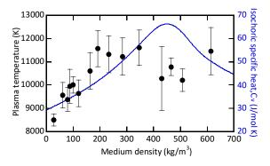
**Figure 9.** Plasma temperature and isochoric specific heat of  $CO_2$  as a function of medium density of  $CO_2$ .
