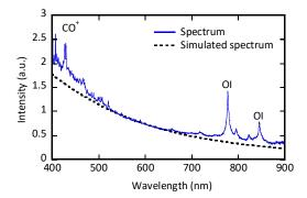
**Figure 8.** Optical emission spectra of pulsed arc discharge measured at ( $\rho = 347 \text{ kg/m}^3$ ) and simulated spectrum on the basis of a Planck's blackbody radiation law.
