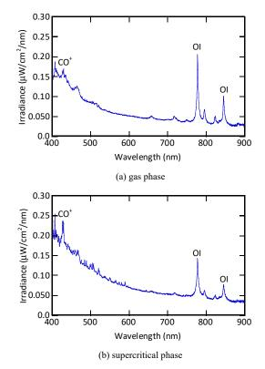
**Figure 6.** Optical emission spectra of pulsed arc discharge under high pressure  $CO_2$ . (a) high pressure gas phase at 61.2 kg/m<sup>3</sup>. (b) supercritical phase at 466.1 kg/m<sup>3</sup>.
