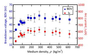
Figure 4. Pulsed breakdown voltage and pulse are current as a function of the medium density of  $\mathrm{CO}_2$
