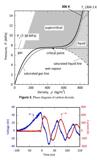
**Figure 3.** Voltage and current waveforms ( $\rho = 347 \text{ kg/m}^3$ ). The first peaks of voltage and current are determined as "breakdown voltage" and "arc current", respectively.
