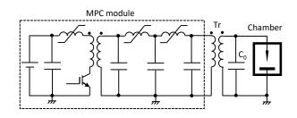
(b) Experimental circuit including MPC module
