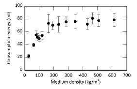
Figure 5. Consumption energy as a function of the medium density of CO<sub>2</sub>.
